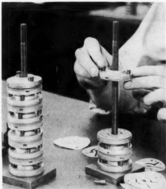
BATCH HANDLING: For convenience, 15 rotor end-plate assemblies are loaded on these center-rod fixtures.
